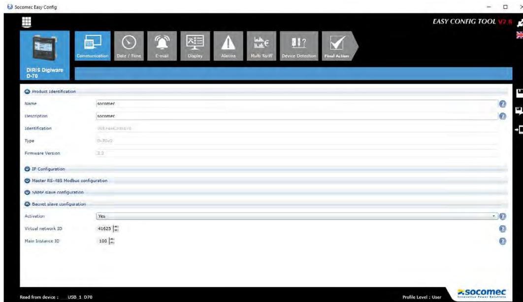
**Activation:** enable or disable the Bacnet IP function
