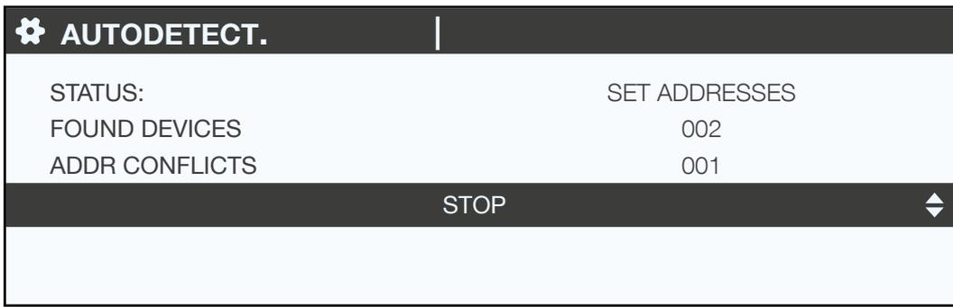
To resolve address conflicts, locate the lit and stable "COM" LED on the front of each product. Press and hold down the addr. button on the front face of the module for a few seconds until the LED flashes:
