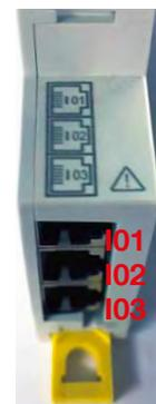
The current sensor connected to the current 1 input measures the current of phase 3 (V3)
